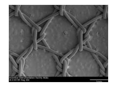
**Polyethylene (PE) LLINs** are typically made from single-filament yarns extruded with additives, colorants, and insecticide. As a result, the insecticide is distributed throughout the yarn, a process known as 'incorporation' technology.
