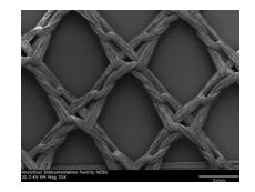
**Polyester (Polyethylene Terephthalate, PET) LLINs** are made from yarns composed of multiple filaments twisted together during the production process. In PET LLINs, the insecticide is applied as a surface coating.
