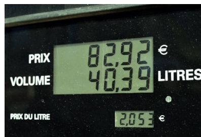
Figure 1 : Illustration of fuel volume measurement at a service station
